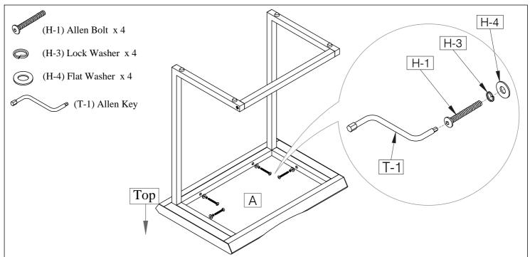
Place Top Panel (A) upside down onto a non-marring surface. Secure the assembled metal base (from Step 1) to Top Panel (A) using Allen Bolts (H-1), Lock Washers (H-3) and Flat Washers (H-4), stacking the hardware in the order as shown. Fully engage all bolts first and then fully tighten using Allen Key (T-1).
