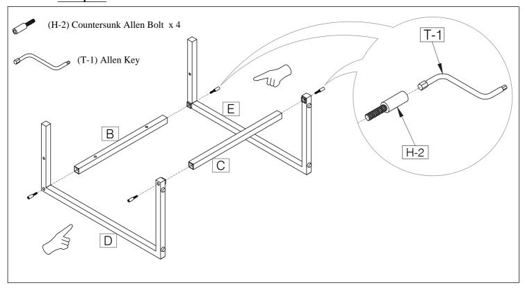
On a non-marring surface, position and secure Top Rail (B) and Bottom Rail (C) to Left Leg (D) and Right Leg (E) as shown. Secure both rails using Countersunk Allen Bolts (H-2). Fully engage all bolts and then fully tighten using Allen Key (T-1).
